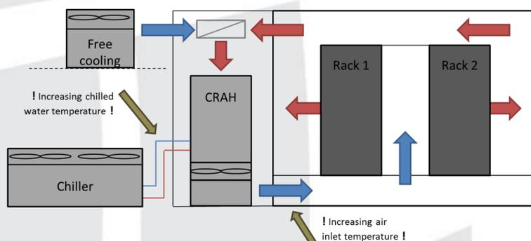
Figure 1. Schema of the cooling system of the data centre.
